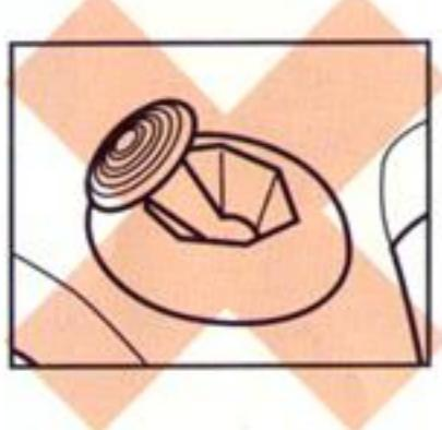
If the Control Stick is held at an angled position (as shown in the picture on the left) when the power is turned ON, this position will be set as neutral. This will cause games using the Control Stick to operate incorrectly.
